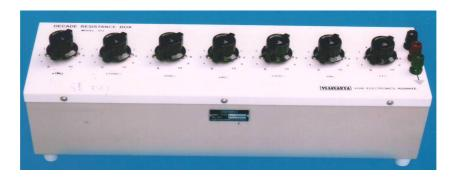
The laboratory quality, low priced decade boxes are designed for maximum usefulness and economy in laboratory measurements testing and development work.
