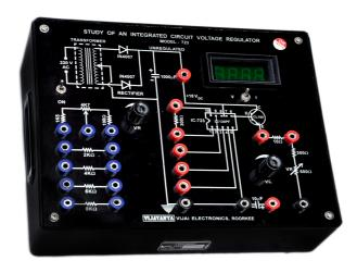
The 723 is a monolithic precision voltage Regulated constructed on a single silicone chip. The device consists of a temperature compensated reference, error amplifier, Power series pass transistor and current limit circuitry. Some of its important features – adjustable output voltage from 2 to 37, Volts of either polarity, 0.01% line and 0.03% load regulation, output current upto 150, mAmp. without external pass transistor make it a general purpose I.C. for voltage or current regulation.
