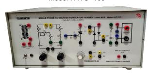
Speed control of AC motor using TRIAC model AVC -109 is very useful in the study and demonstration of the principle and working of a Speed control of AC motor. Student understand the firing method of TRIAC and speed control of AC motor different firing method. Multi colored Test Points are provided at various stages in the circuit to observe the waveforms and voltages. It is strongly supported by a comprehensive Instruction Manual complete with theory and operating details.
