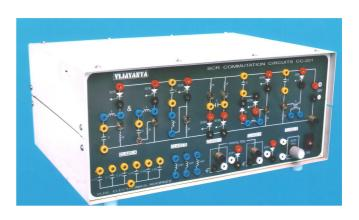
All cares have been taken to make this unit convenient, simple in working. The commutation unit is fully self content. Only a general purpose C.R.O. and multimeter are required to perform experiments. All key components are mounted on a glass epoxy P.C.B.
