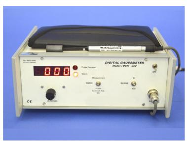
magnetic field. The magnitude of this e.m.f. is proportional to the field intensity if the current is kept constant.
