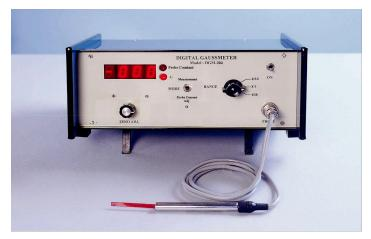
when placed in a magnetic field in a direction perpendicular to the direction of both electric current and magnetic field. The magnitude of this e.m.f. is proportional to the field intensity if the current is kept constant. This e.m.f. is called the Hall Voltage. This small Hall Voltage is amplified through a high stability amplifier so that a milli voltmeter connected at the output of the amplifier can be calibrated directly in magnetic field unit (gauss).
