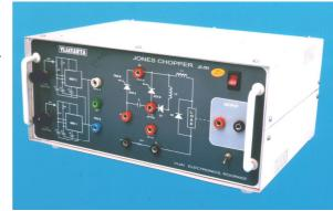
auxiliary SCR. Which is used to turn off the main thyristor. Choppers are very widely used in electric traction, trolley cars, mine hailers, D.C. Voltage regulators, marine hoists etc.
