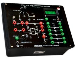
The term Operational Amplifier (Op - Amp.) refers to high gain D.C. Amplifier that has a different input (Two input leads) and a single ended output (One output leads) Op - Amps have characteristics such a high input resistance, low output resistance, high gain. Low drift etc. that make them highly suitable for many application and therefore, wide spread use in electronic circuit.
