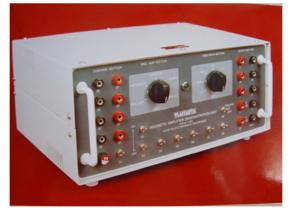
This is a very versatile unit which can be used for performing different experiments just by means of selector switches. All the control characteristics of basic transductors and Magnetic amplifier can be studied. The following gives a list of experiments that can be performed with this demo unit :
