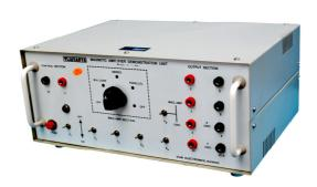
This is a very versatile unit which can be used for performing different experiments just by means of selector switches. All the control characteristics of basic transductors and Magnetic amplifier can be studied. The following gives a list of experiments that can be performed with this demo unit
