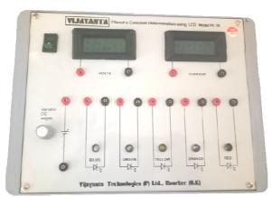
**PC-10 Planck's Constant determination using LED** is a useful setup which illustrates the basic concept of the Quantum Mechanics. The setup familiarizes the concept of photon energy and explains how it is related to its frequency. Setup is mainly designed to evaluate Planck's Constant. For this purpose five LEDs of different colors are included with the setup. This setup facilitates to determine the Planck's Constant by measuring the voltage drop across LEDs.
