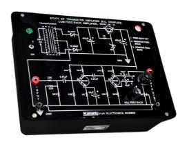
This is a two stage transistor amplifier with a provision for positive and negative feedback. The amount of feedback is adjustable and with the help of this it is even possible to make the amplifier oscillate. A 9, Volts stabilized power supply is provided on the same board.
