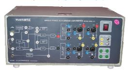
The phase controlled converter can operate either in rectification mode or in inversion mode. In rectification mode, AC power is converted to DC power and in inversion mode DC power is converted to AC power. The unit is capable to operate in both modes.
