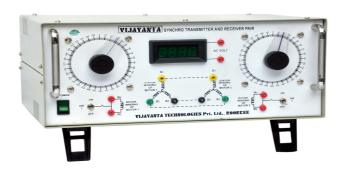
The system set up is made up of synchro transmitter and synchro receiver on a single rigid base provided with suitable switches and anodized angular plates. The system also contains a step down transformer for providing excitation to the rotors.
