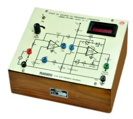
This board is designed to study of an operational amplifier working as voltage to frequency converter. The board is fully self contained hence no other apparatus required to perform the experiments. The board has one  $Op-Amp\,\mu A-741$  with four resistors of same values, one continuously variable D.C. Supply 0-15, Volt and one Voltmeter, sockets provided for connections and necessary number of patch (cords) leads provided with board.
