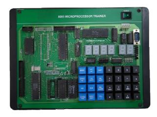
VTPL-8085 is a single board Microprocessor Trainer Kit based on 8085 Microprocessor which is widely used to train engineers to develop software / hardware for any industrial process & control. This Kit consists of power-full Monitor EPROM, RAM, I/O Lines, Timer/Counter, Serial, Seven Segment Display and Keyboard for Man to Machine Interface.
