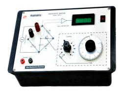
The Anderson Bridge is usually used for measurement of Inductance in terms of Capacitance and Resistance. The actual circuit is printed on the panel. A builtin 1 KHz Since Wave Frequency Generator. Tuned frequency amplifier as Null detector and a moving coil Microamperemeter for Null indication & the Power Supply all are builtin. Thus these Bridges are self contained and also complete in all respects. Fitted with a pair of terminals. Marked "Phone / CRO" to be used with Headphone or C.R.O.
