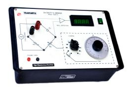
This Bridge was specially developed to measure capacitance having low 'D' factor. The 1 KHz Oscillator and tuned amplifier fitted with Moving Coil Micro Ampere Meter as Null Indicator and power supply are builtin.
