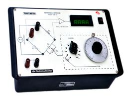
The Maxwell Bridge is generally used for the measurement of low "Q" self Inductance for which "Hay" equation have awkward characteristics. It is not so desirable for high "Q" coils as it requires large values frequently inconveniently for R1 and does not give a sharp resistance unknown inductance. Null detector with builtin 1 KHz Oscillator. A digital meter for Null Detector and a D.C. Microamperemeter for Null Indication. The actual bridge and formula is given in operating instructions.
