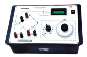
Schering Bridge is one of the most important A.C. Bridge. It is used in the measurement of capacitance in general. The Schering Bridge circuit is basically the same as capacitance comparison bridge. The basic circuit and formula are engraved on panel. Terminals are fitted for connecting headphone and unknown capacitance. The 1 KHz Oscillator and tuned amplifier with Micro Ampere Meter as Null Indicator and Power Supply are builtin.
