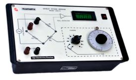
The specialty of this bridge is that its measures resistance in wide range of DC or AC both. Terminals are provided to connect headphone and unknown resistance. 1 KHz Oscillator and tuned amplifier with Moving Coil Micro ampere Meter as a Null Indicator and power supply are builtin.
