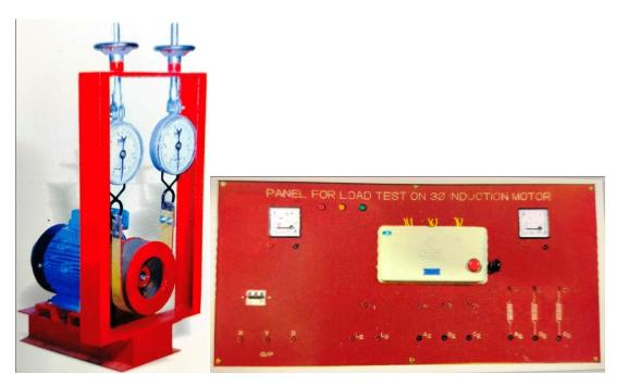
AC Squirrel Cage Motor with pony brake loading arrangement with dial type spring balance with control panel. Technical Specification: A.C. SQUIRREL CAGE INDUCTION MOTOR2 HP WITH DOL / STAR DELTA STARTER with Mechanical Load - AC MOTOR:- It should be A.C. 3 Phase 2HP 415 volts, 50 Hz, Efficiency – 86.3% on full load Squirrelcage Induction Motor, horizontal foot mounted.
