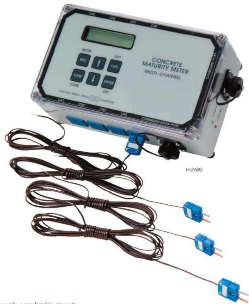
Maturity Meters provide a predictable strength determination of cast-in-place concrete based on ASTM Standard C1074-98 (Estimating Concrete Strength by the Maturity Meter Method). These units utilize inexpensive, disposable, T-type thermocouple wire with quick-connect jacks, which can be embedded directly into a concrete structure to measure temperature at timed intervals. These readings can then be used to document the maturity process within the structure in order to:
