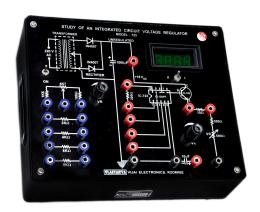
The 723 is a monolithic precision voltage Regulated constructed on a single silicone chip. The device consists of a temperature compensated reference, error amplifier, Power series pass transistor and current limit circuitry. Some of its important features – adjustable output voltage from 2 to 37, Volts of either polarity, 0.01% line and 0.03% load regulation, output current upto 150, mAmp. without external pass transistor make it a general purpose I.C. for voltage or current regulation.
