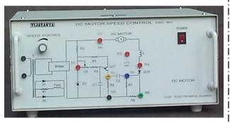
All components are mounted on a glass epoxy PCB. Basic block diagram is printed are brought out to the banana sockets mounted o front panel for observations.
