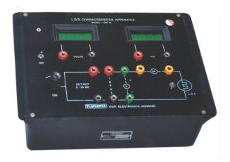
Study of L.D.R (Light Dependent Resistance) Characteristic Apparatus has been designed to draw the characteristic curve between Resistance and Light Intensity at different voltages.
