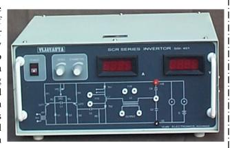
All components are mounted on glass epoxy PCB. Basic block diagrams is printed on the front panel and all test points are brought out to the banana sockets mounted on front panel for observations.
