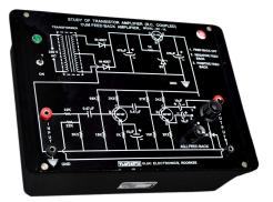
This is a two stage transistor amplifier with a provision for positive and negative feedback. The amount of feedback is adjustable and with the help of this it is even possible to make the amplifier oscillate. A 9, Volts stabilized power supply is provided on the same board.
