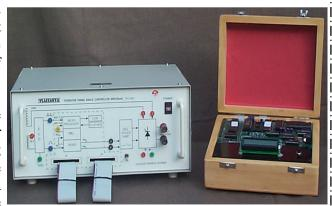
Four thyristors are connected in a bridge form with suitable heat sinks & snubber circuits for protection.
